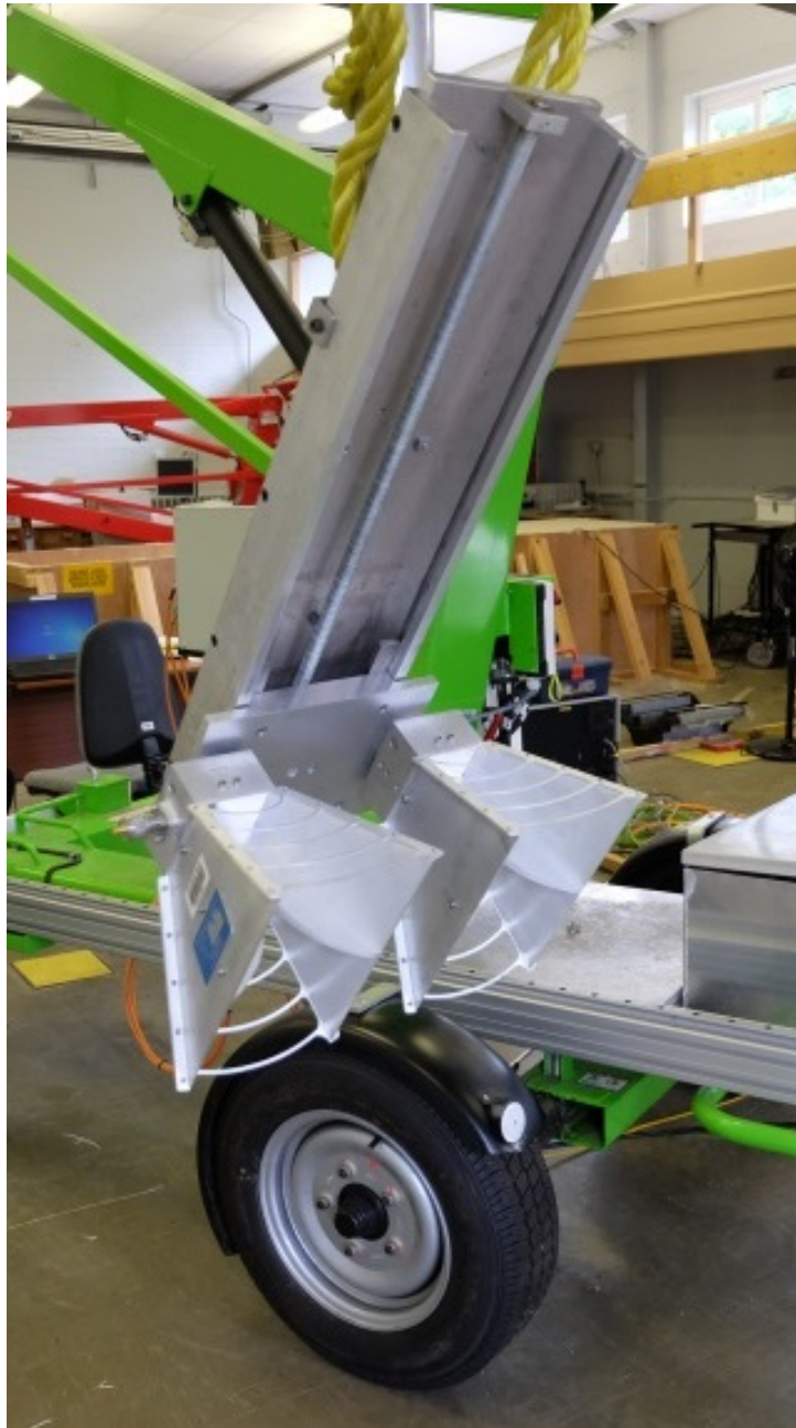
Figure 1: Radar Interferometry mount repurposed for the collection of accurately aligned 2D apertures for 3D SAR image formation. The broadband horn antennas were mounted on the interferometer hand-wound mechanism.
