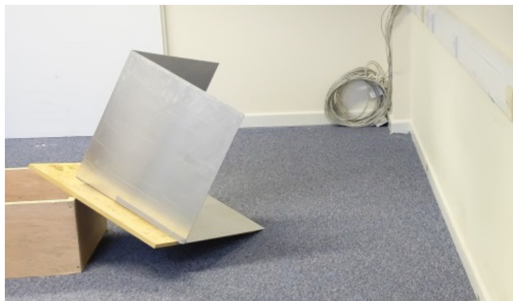
Figure 3: Radar-far-side of concrete wall measured scene showing the large 600mm trihedral target.
